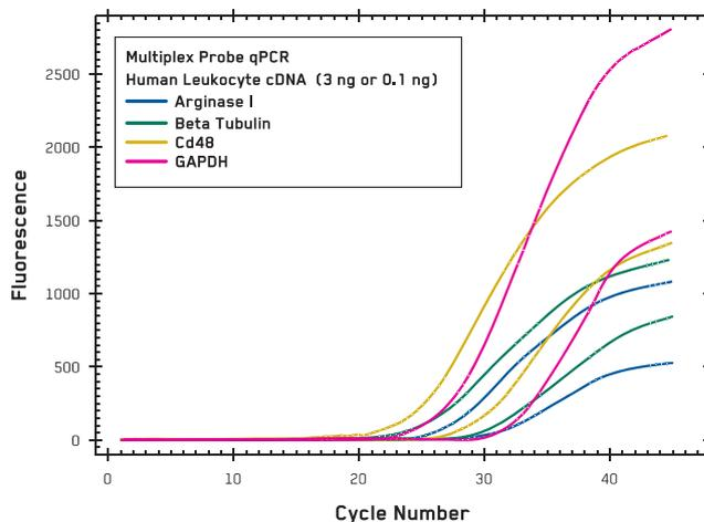
**Figure 1:** Probe-based real-time PCR plus UNG pretreatment with EURx M<sup>3</sup> Multiplex Master Mix - Probe qPCR (= MP Probe qPCR Master Mix), specific primers and fluorescent labeled probes binding within the amplicon (FAM, HEX, Texas Red, Cy5). Reactions were performed by using human leukocyte cDNA (3 ng or 0.1 ng) as template. Measured PCR efficiency was greater than 85%.
